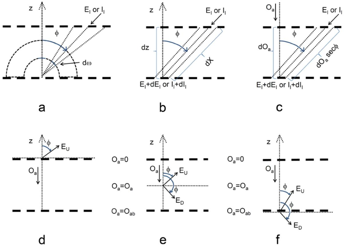
Figure 3.15. Geometry and notation used by the radiative-equilibrium and radiative-convective models.
