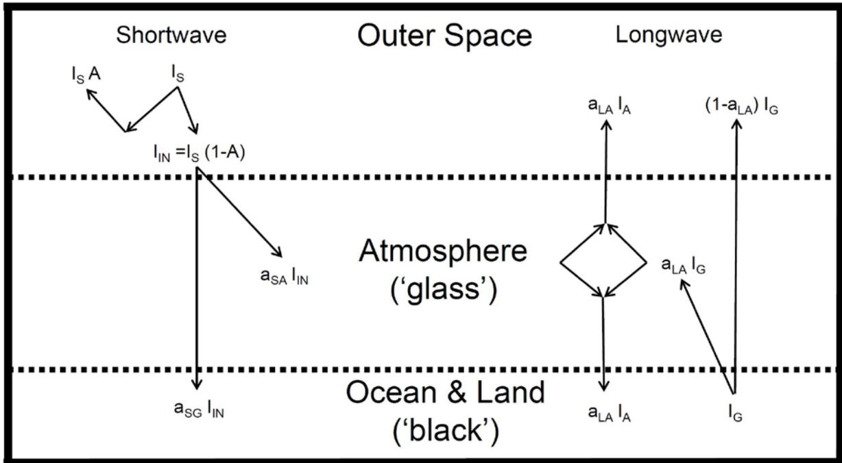
Figure 3.5 Parameters for the 'glass slab' model of radiative balance for the global atmosphere.
